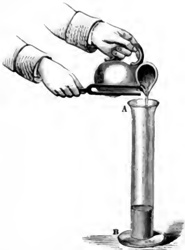
FIG. 46 (Tyndall). Representing water being poured into the vessel A B, till the air-space is just sufficient to respond to the vibrations of the tuning-fork. The air thus becomes a resonator of the fork.
